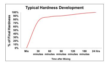
If the cure time needs to be reduced and after WRM Premium has been applied to the damaged area, hot air blowers or heated enclosures at temperatures from 60°C-80°C may be used to accelerate the cure and property development.
